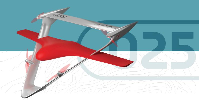
The FIXAR 025 is an autonomous fully electric drone designed to handle large-scale and long-range missions for commercial and industrial applications, such as mapping and inspections, aerial imaging, remote sensing, surveillance, monitoring, and more.
